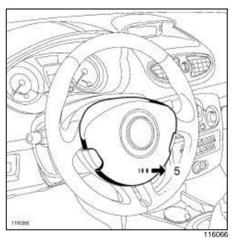
❑ Apply pressure (4) on the clip using the T-bar with the extension, whilst slowly pulling the airbag module towards you (5) to unclip the lower section of the airbag.
