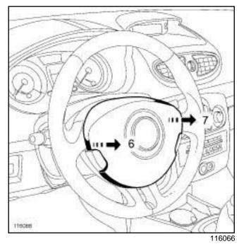
□ Unclip the airbag module connector at (6) and (7).
