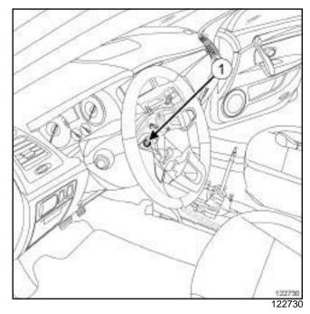
□ Remove the steering wheel bolt (1).
